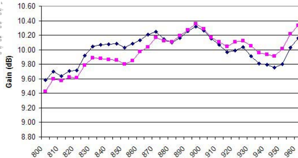
Fig.8 Measured Gain on two polarizations
