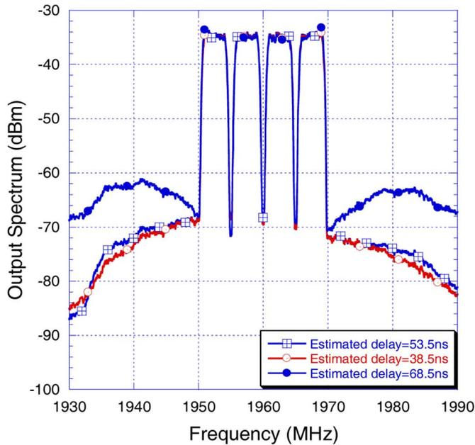
Fig. 3. Model output spectra (delay estimation error = 15 ns).
