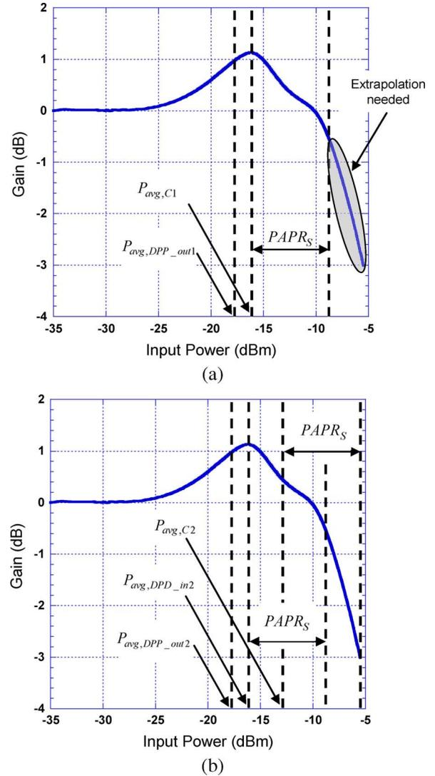
Fig. 3. Power levels at characterization and linearization steps. (a) Constant average power approach. (b) Constant peak power approach.
