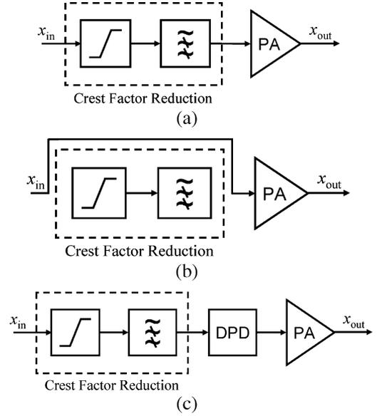
Fig. 4. Block diagram of the transmitter configuration for: (a) conventional PA characterization, (b) proposed PA characterization, and (c) PA linearization.
