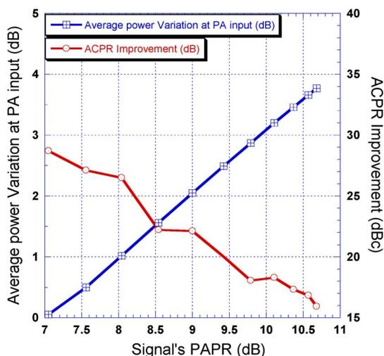
Fig. 6. Measured ACPR improvement at the output of the linearized PA, and average power variation at the PA input.
