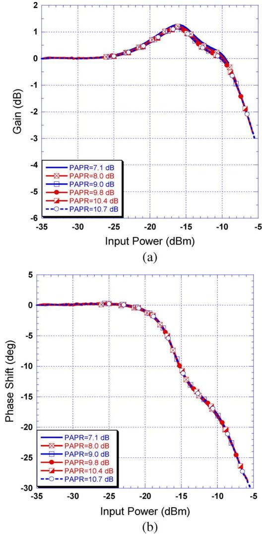
Fig. 2. PA's measured characteristics at constant average input power levels. (a) AM/AM characteristics. (b) AM/PM characteristics.
