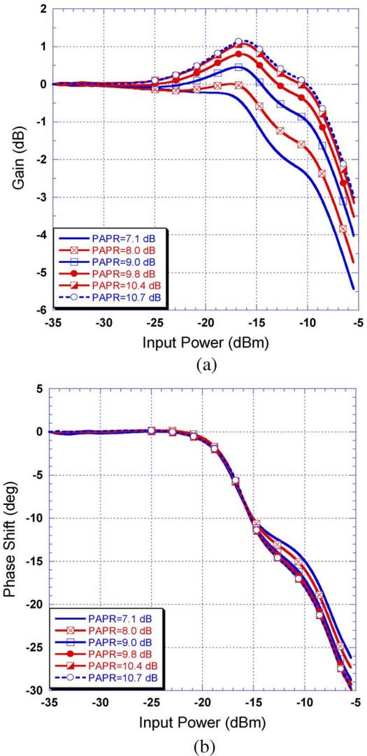
Fig. 1. PA's measured characteristics at various average input power levels. (a) AM/AM characteristics. (b) AM/PM characteristics.
