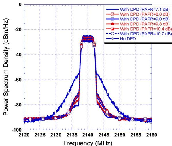
Fig. 5. Measured spectra at the output of the linearized PA.
