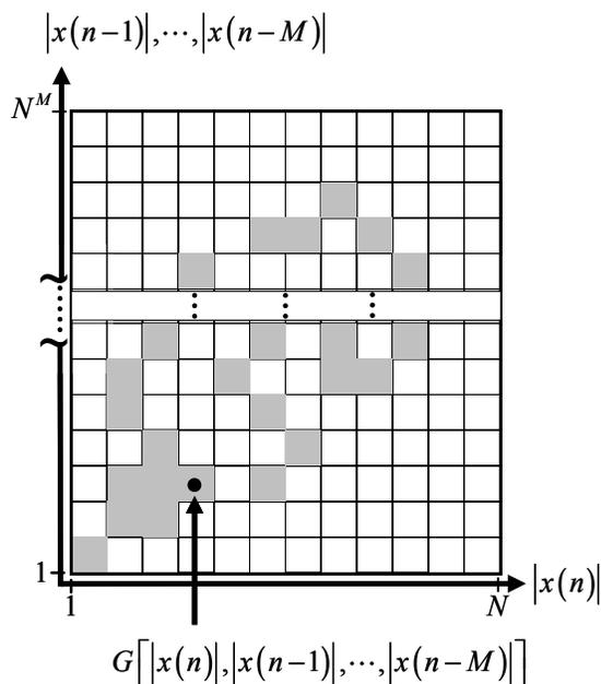
Fig. 1. Block diagram of the 2-D LUT model.
