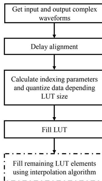
Fig. 3. Flow chart of the model identification process.
