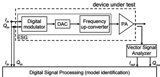
Fig. 2. Measurements setup used for experimental validation.
