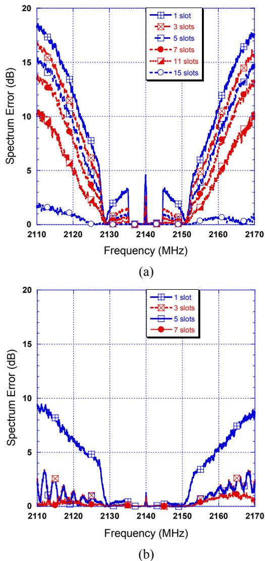
Fig. 5. Frequency domain error. (a) without interpolation, (b) with interpolation.
