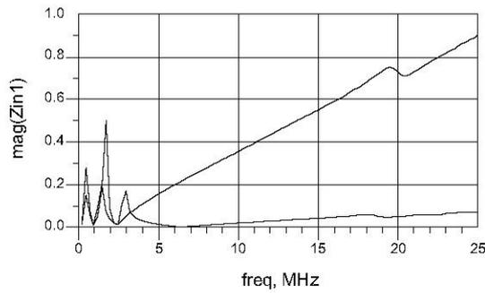
Fig.3. The video impedance of the output network with and without  $C_{18}$  and  $C_{19}$  decoupling capacitors.
