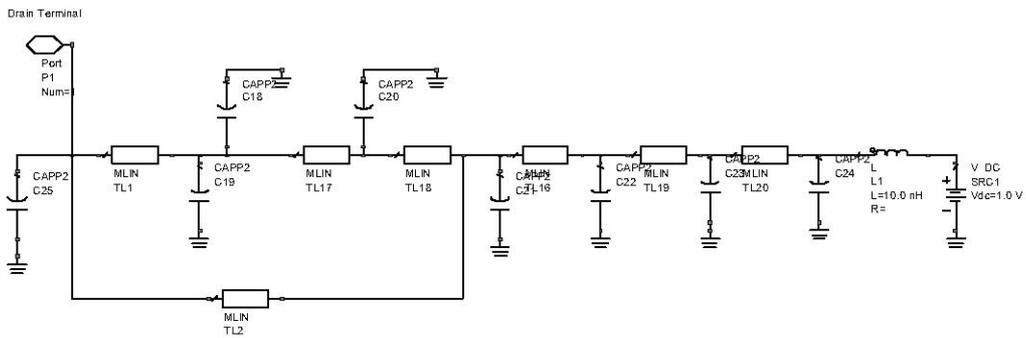
Fig 2. Typical implementation of bias circuitry designed for high power application.
