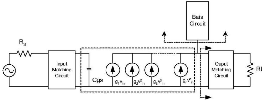
Fig. 1. Typical amplifier circuit representation with nonlinear trans-conductance model.
