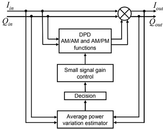
Figure 1. Functional block diagram of the proposed predistorter
