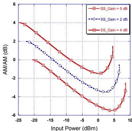
Figure 2. DPD's AM/AM characteristics vs. its small signal gain
