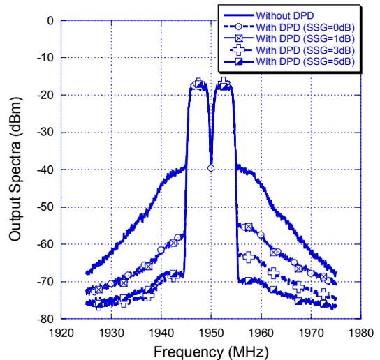
Figure 3. Measured spectra at the output of the PA vs. DPD's small signal gain
